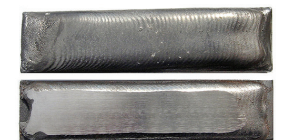
Double pass overlays welded onto A36 steel with 73.1 HRC average
